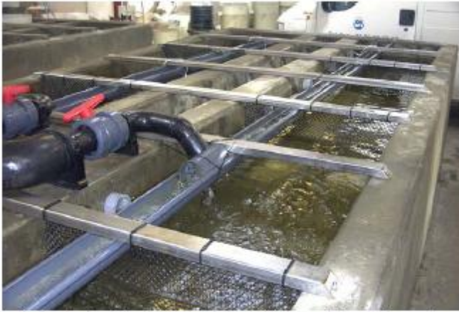
Figure 7.2 Distributed by two long tanks were razor mussels established in 10 units with an area of 1.0 × 0.5 m. Between the units that were tagged with networks, there was free water exchange. The water was distributed throughout tank using a gutter with holes.
